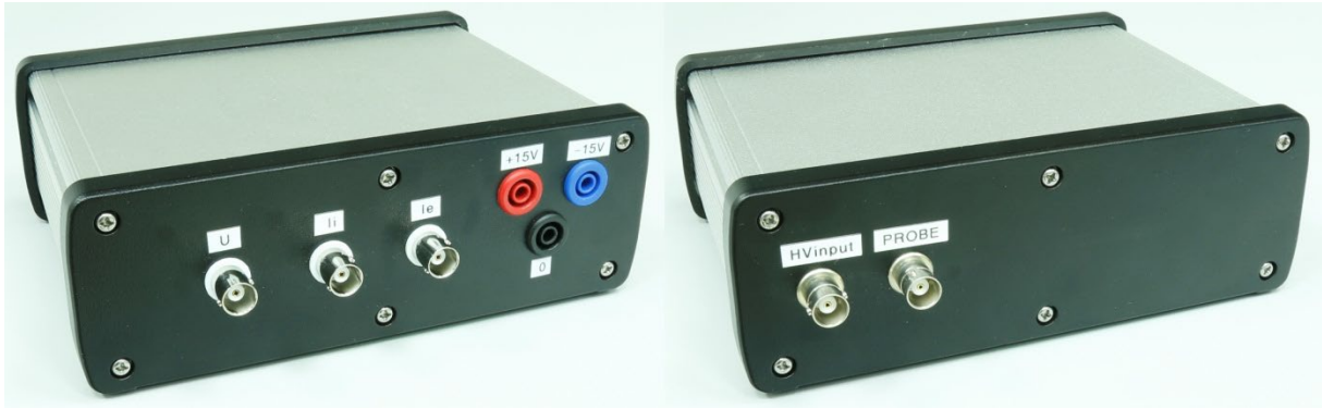
Figure 9. First version of acquisition electronics. On the left hand side are three isolated measurement channels and power supply input. On the right hand side are input for HV biasing signal and probe connection.
