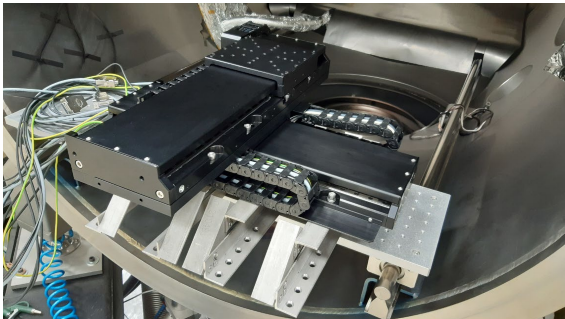
Figure 16. XY manipulator on top of the scaffolding during installation in the vacuum chamber. The scaffolding is fixed both to the new optical breadboard (in the picture) and to the old one with the thrust balance and the thruster (not yet visible in the picture).
