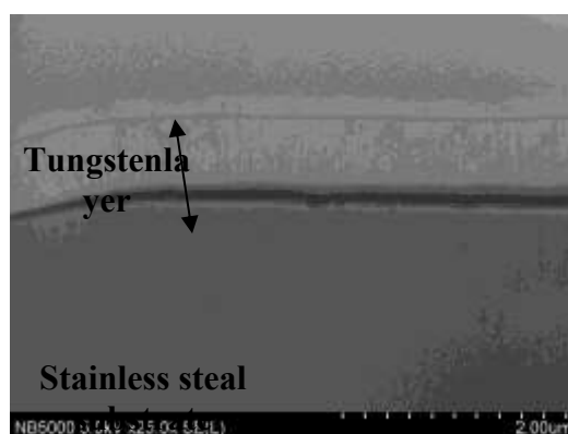
Fig.3. A cross-section of the tungsten layer, sample2, polished side
