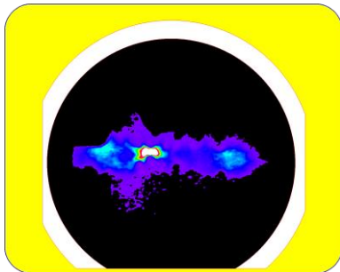
Fig.3 The image of hot plasma emitting soft X-ras recrded on a phosphor screen of MCP based camera
