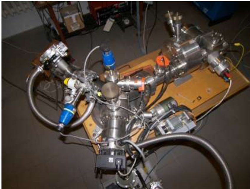
Figure 1 W7-AS X-Ray Monochromator with implemented X-Ray Tube
