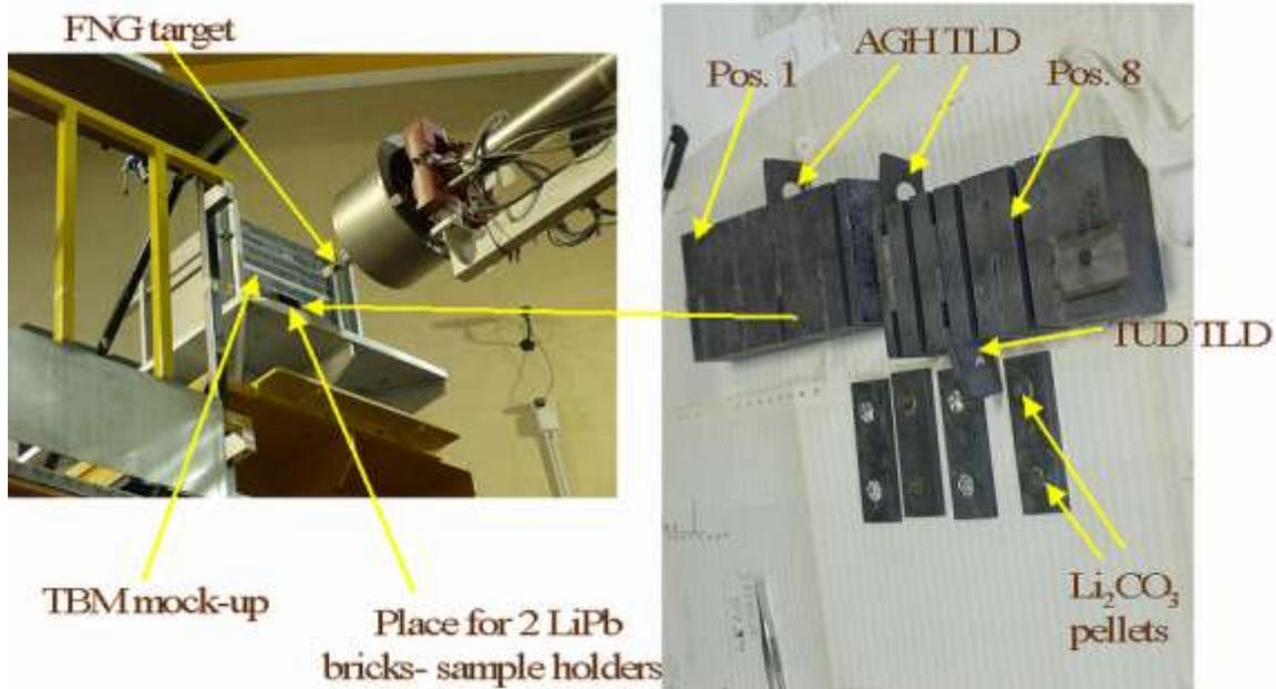
Figure 1. TBM HCLL mock-up in ENEA Frascati FNG Laboratory
