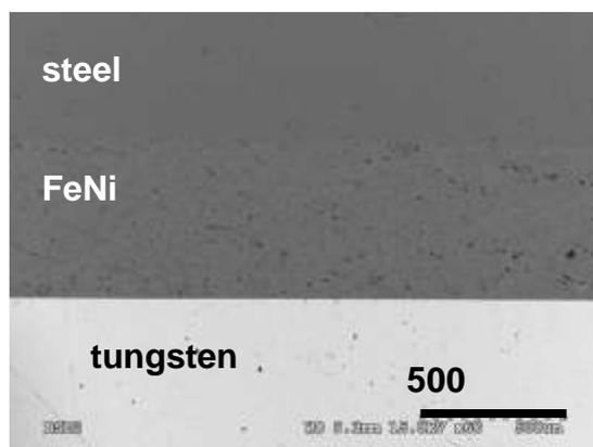
**Figure 3.** SEM image of the W/FeNi/steel joint cross section
