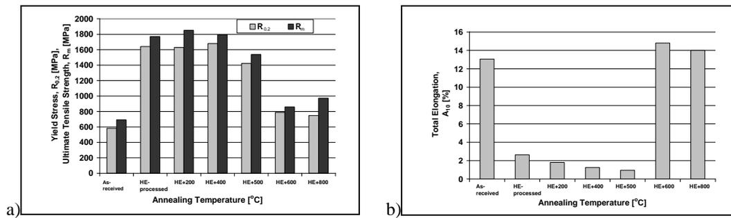
**Figure 2** Ultimate Tensile Stress  $R_m$  Yield Stress  $R_{0.2}$  (a), Total Elongation A(b)
