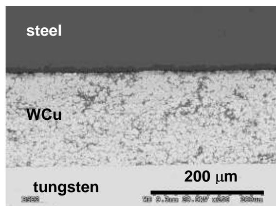
**Figure 1.** SEM image of the W/W+Cu composite/steel joint cross section
