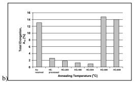
Figure 2 Ultimate Tensile Stress R<sub>m</sub> Yield Stress R<sub>0,2</sub> (a), Total Elongation A(b)
