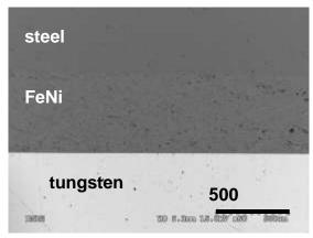
Figure 3. SEM image of the W/FeNi/steel joint cross section
