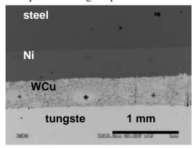
Figure 2. SEM images of the W/WCu composite/Ni/steel joint cross section
