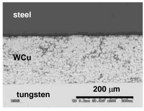
Figure 1. SEM image of the W/W+Cu composite/steel joint cross section
