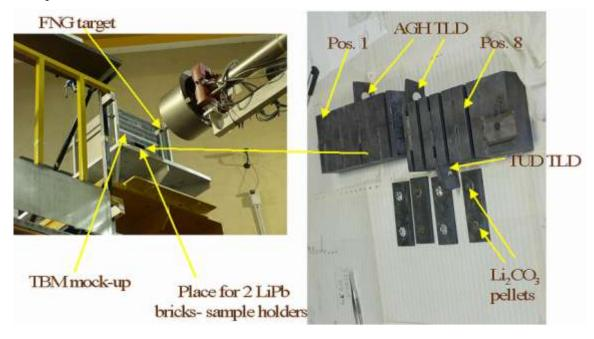
Figure 1. TBM HCLL mock-up in ENEA Frascati FNG Laboratory
