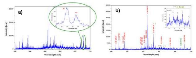
Figure 2 a) a sample spectrum obtained for virgin codeposit with highlighed deuterium line b) a spectrum of a cleaned surface
