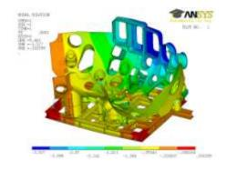
**Figure 6.** Vertical displacements of the transportation system with a lower shell
