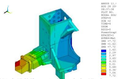
Displacements (USUM) in the NPC1-Z2connection; Bolts preload at 4 K and operational loads - step 4; Load case LS(45)
