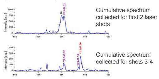
**Figure 1** Evolution of spectra of a AUG sample during first 4 laser shots – presence of deuterium line is clearly visible for the first 2 shots.
