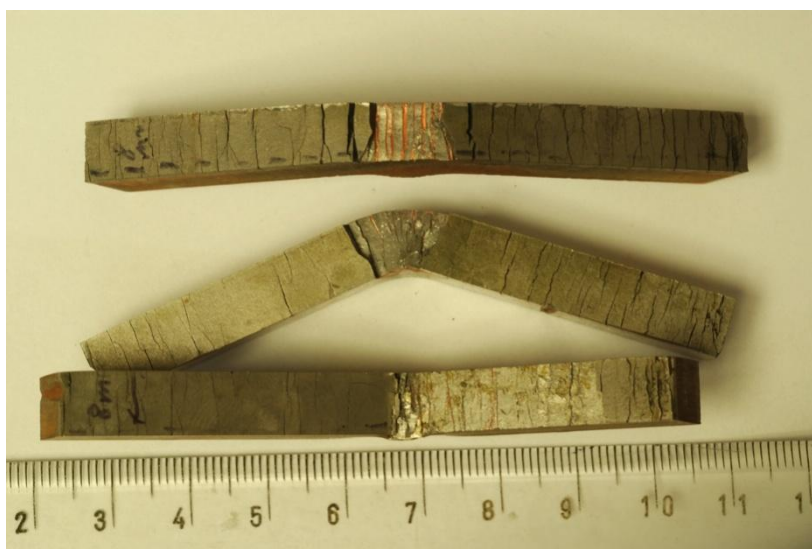
Fig. 2 Tungsten-to-steel joints produced by explosive bonding after bending tests
