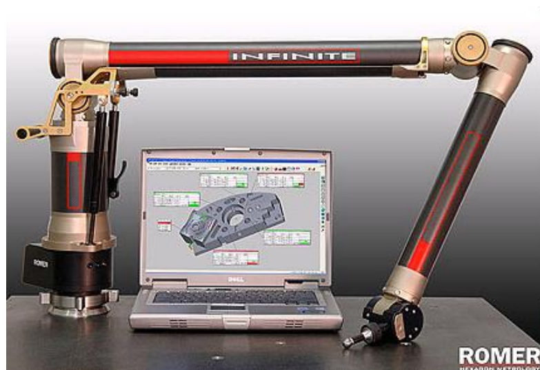
Fig. 1 An arm for laser scanning inspection system provided by ROMER
