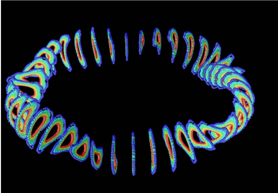
Calculated 3D electron temperature solution in a W7-X configuration
