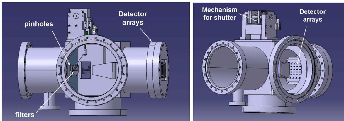
Design of the MFS soft X-ray diagnostic system for W7-X done by the IPPLM, Warsaw.
