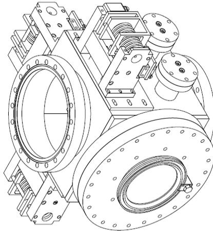
Vacuum chamber of PHA soft X-ray diagnostic designed and built at the IPPLM, Warsaw for W7-X stellarator.
